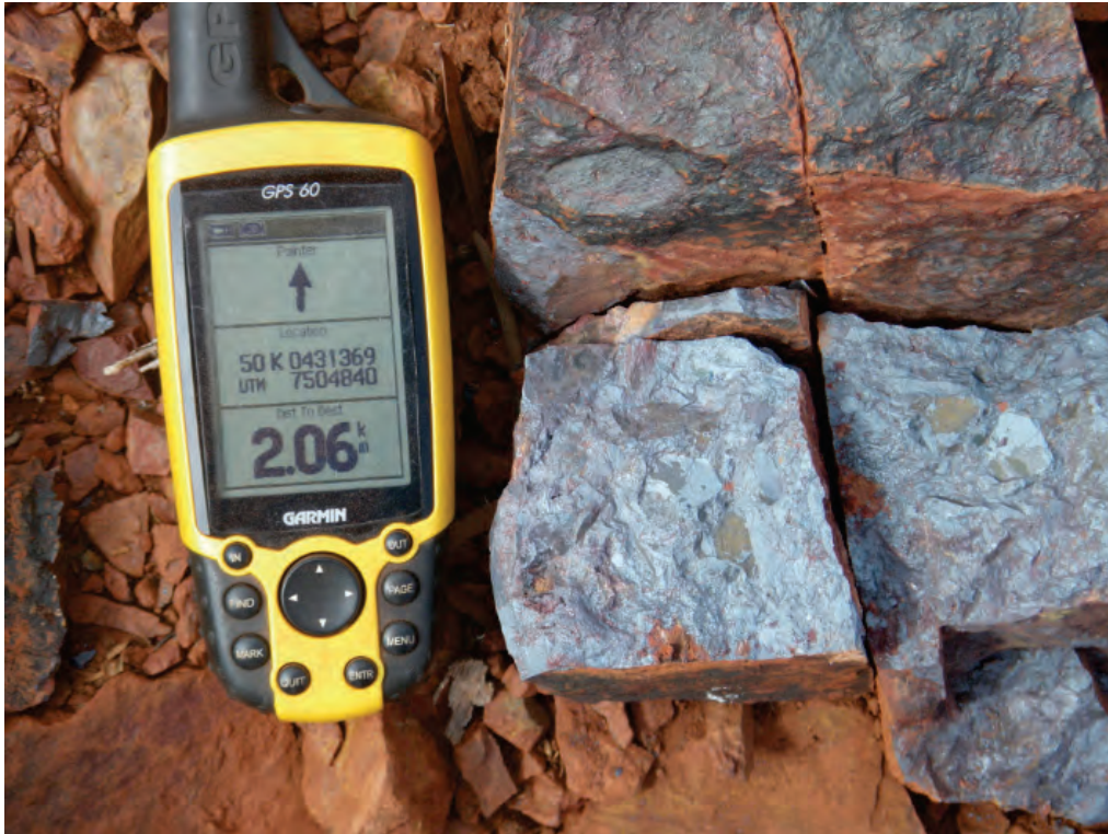
Figure 17: Close up view of hematite conglomerate with hematite matrix as found at Paulsens East
